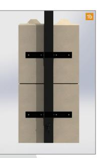
**1Double Block Setup:** Position the straps approximately halfway up the face of each block.
