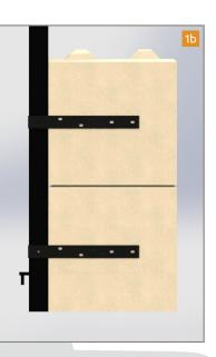
**1Double Block Setup:** Position the straps approximately halfway up the face of each block.
